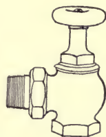
IMPROVED VALVE FOR STEAM RADIATOR.
