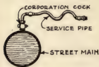
FLEXIBLE CONNECTION TO STREET MAIN.
