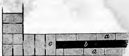
[Fig. 4. Hollow 8 inch wall.]
